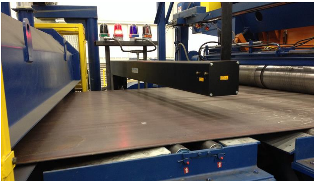
AGT800 Thickness Gauge operating on a 96" Stretch Leveler Line
